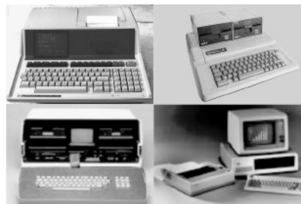
Figure 4. Examples of early desktop PCs, HP85 (a), Apple II (b), Osborne (c) and the first IBM PC (d).
