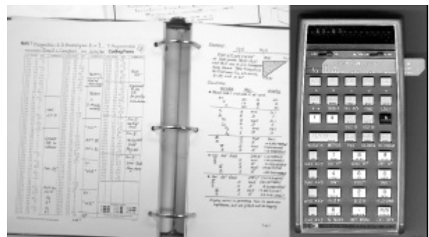
Figure 3. SEG programs for the Texas Instruments 59 calculator and an image of the HP 67 hand held programmable calculator.
