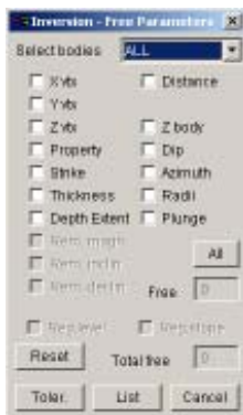
ModelVision Pro inversion control panel provides access to any body parameters in any and all bodies in the model
